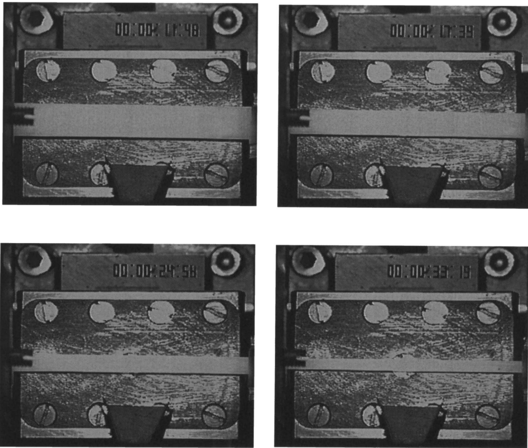
Figure 2 Images of sample deformation in four selected steps at strain rate of 0.1 (1/s), and temperature of 150 °C. Homogenous deformation can be observed.
